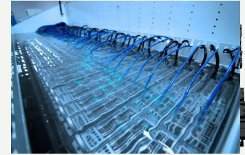
Example of immersion cooling of server racks
